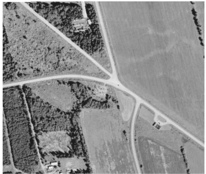
Figure 2: A Before and After view of a five-way intersection in rural Prince Edward Island. In the After situation (shown in the right-hand image), the northbound approach has been realigned to meet with the through road east of the intersection. This example shows an imperfect solution to the problem, since two other legs still intersect at skewed angles, and the design also allows for serious movement conflicts. This was presumably deemed acceptable by the local authority due to the very low volumes on the minor legs. (Courtesy: Province of Prince Edward Island)
