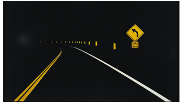
Figure 6: Use reflective markings for nighttime visibility where the rural intersection is not serviced by overhead lighting. Note the advisory speed tab used in conjunction with the warning sign. Note also that this illustration does not necessarily indicate an intersection.
