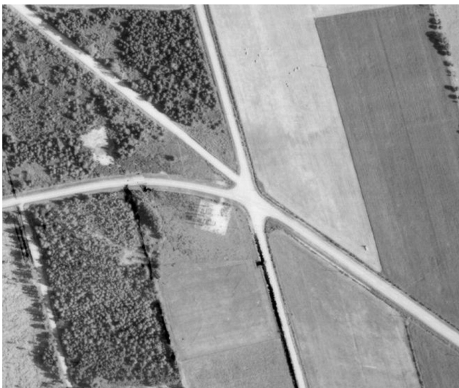
Figure 2: A Before and After view of a five-way intersection in rural Prince Edward Island. In the After situation (shown in the right-hand image), the northbound approach has been realigned to meet with the through road east of the intersection. This example shows an imperfect solution to the problem, since two other legs still intersect at skewed angles, and the design also allows for serious movement conflicts. This was presumably deemed acceptable by the local authority due to the very low volumes on the minor legs. (Courtesy: Province of Prince Edward Island)
