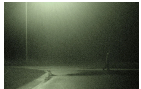
Figure 3: Pedestrians are much more visible when roadway lighting is installed.
