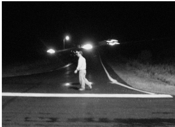
Figure 1: Lighting is generally not cost effective in rural applications. It may be justified however where pedestrians are frequent or where the nature of collisions indicates that there is a problem with conspicuity of the intersection at night.
