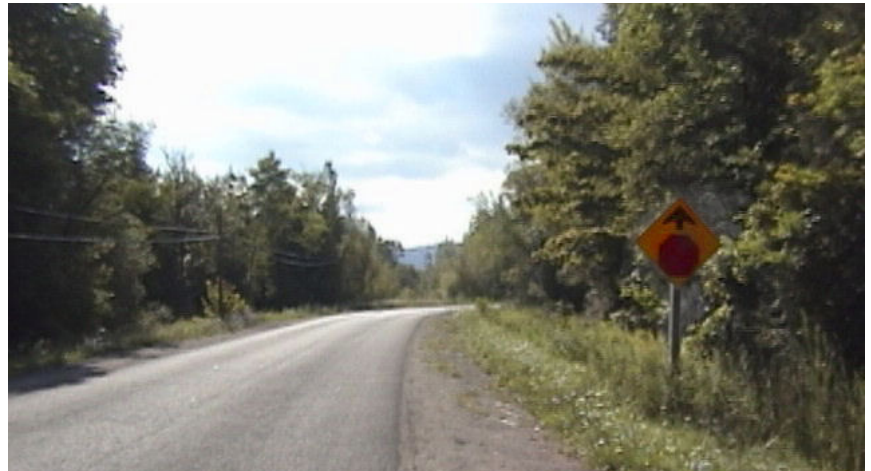
Figure 2: In the photo at the right, an advance warning sign (Stop Ahead) has been used because the sight-lines to the intersection are hidden by vegetation on the inside of the horizontal curve.
